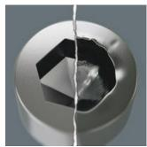
Hexagon screws can endure a problem because the contact surfaces delivering the power from conventional the tool, transferred to the screw via very small surface areas. The consequence: the screw can become damaged (rounding out). Hex-Plus tools have a greater contact surface that prevents this from happening! At the same time, as much as 20 % more torque can be applied. Good to know: Hex-Plus tools fit into every standard hexagon socket screw!
